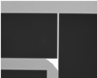
Fig. 4.16 (left) Under-etching at the corner of an L-spring with an etch protecting strip. Dark areas are open parts of the wafer. Dark grey is silicon nitride with silicon immediately underneath; light grey is floating, transparent silicon nitride.
